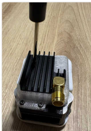
B • Press straight down with a thin screwdriver or a SIM tool.
