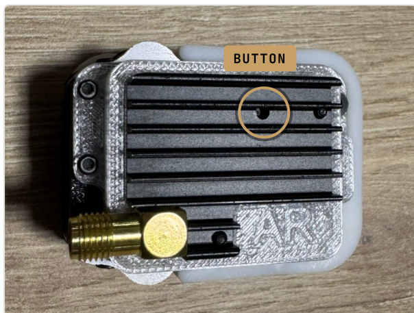
A • The button sits at the bottom of a small hole in the finned heatsink — not the larger hole nearer the antenna socket.
