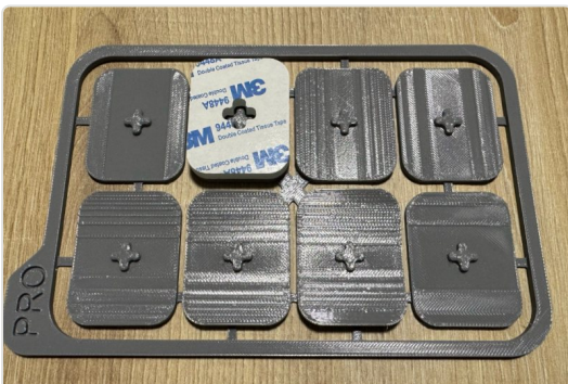
C · Eight pads, eight curvatures, on a frame marked PRO. One shown with its double-sided tape.
