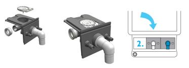
**3.** Check **expiratory flow sensor** for correct assembly and install.
