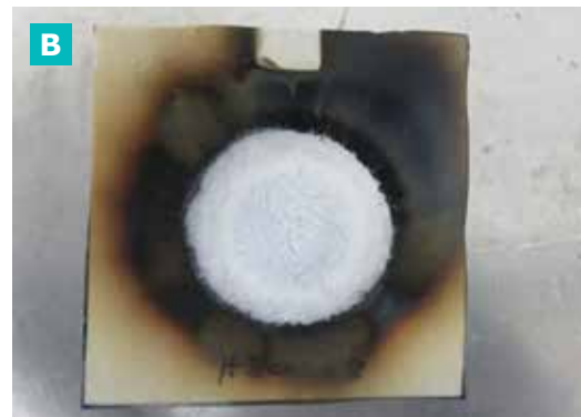
Figure 20: UP-laminate (15 wt.-% GF) after torch test: A) 300 phr APYRAL® HC 500 and B) 200 phr ACTILOX® HTB .
