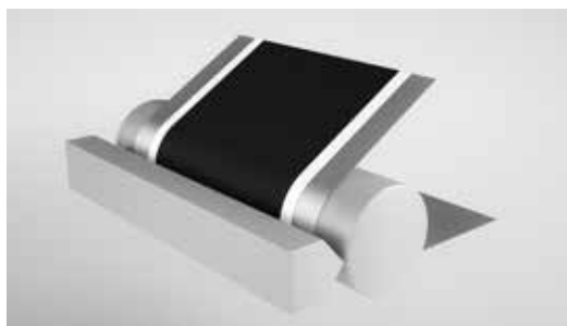
Figure 4: A die coating system in which the boehmite dispersion is applied to the cathode edge.
