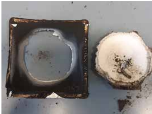
PA6_5%GF_50% ACTILOX® HTB -a 15 min until solid, ceramic like residue breaks out
