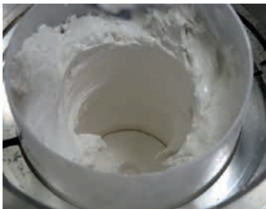
Figure 11: Aborted experiment trying to disperse 27 vol.-% of BN in UP-resin. All material clogs to the wall while the dissolver blade (not shown) is mixing only air.
