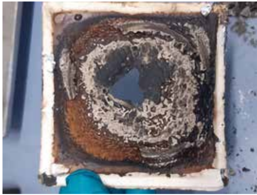
PA6_5%GF_50% APYRAL® AOH 30 4 min until sample burns through
