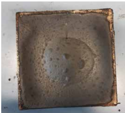
PA6_20%GF_40% ACTILOX® HTB -b No burn through within 20 min; very solid, ceramic like residue; backside temperature < 400 °C
