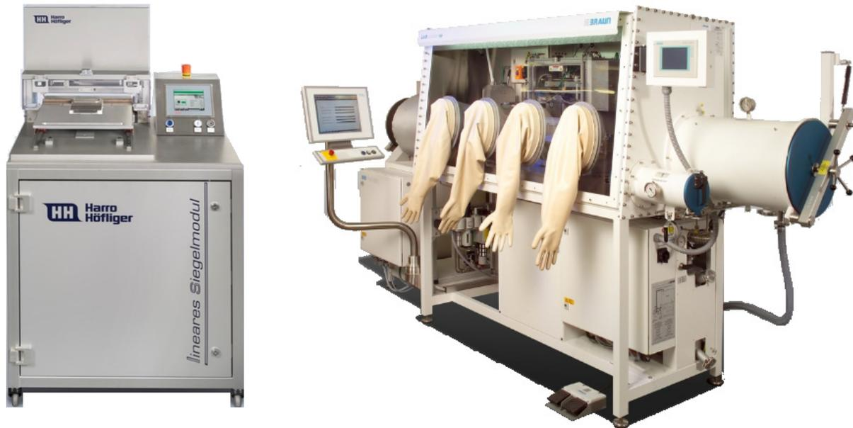
Sealing module (left) and glovebox with integrated vacuum filling and sealing station by Harro Höfliger (right) for semi-manual, highly flexible manufacturing of single- to multi-layer pouch cells at industry-related standards.
