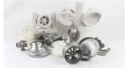
Figure 1. Rapid production of metal parts using PolyCast™ and 3D printing
