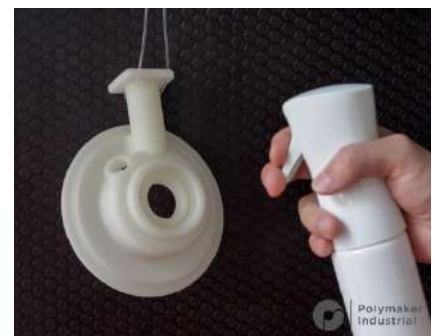
Figure 5. Spray isopropyl alcohol on the PolyCast™ pattern
