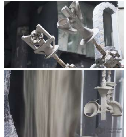
Figure 7. Make the ceramic shell
