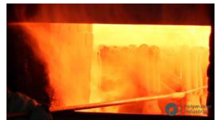
Figure 8. Sinter the ceramic shell and burnout
