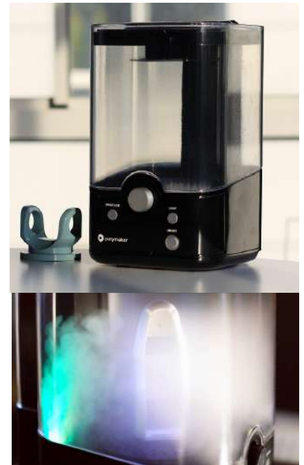
Figure 3. Polish the PolyCast™ pattern by Polysher™
