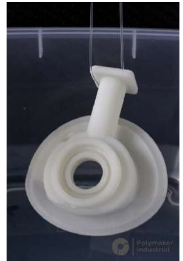
Figure 4. Dip the PolyCast™ pattern into isopropyl alcohol
