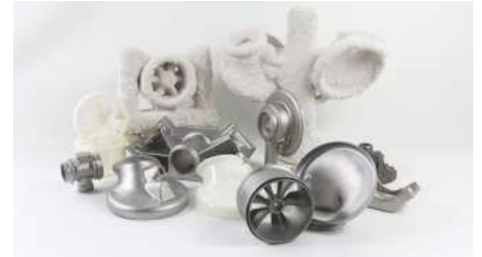
Figure 1. Rapid production of metal parts using PolyCast™ and 3D printing
