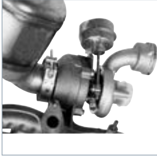
Automotive: Turbocharger – catalytic converter connection
