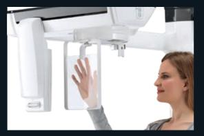
**CARPAL** The teleradiographic module includes a convenient support for carpal scanning.
