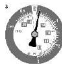
(3) READING: Extremely low but steady DIAGNOSIS: leaking intake manifold system, Faulty manifold gasket or carburettor base gasket, split vacuum hose, seized open EGR valve.
