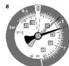
(8) READING: Regular drop Between normal and low reading. DIAGNOSIS: Burnt valve.
