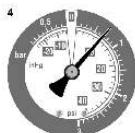
(4) READING: reading low but steady DIAGNOSIS: Retarded ignition timing. Confirm using timing light and reset to manufacturer's specification.
