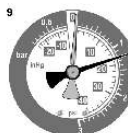
(9) READING: Normal when First started but drops rapidly when RPM held at 3000. DIAGNOSIS: Restriction in exhaust system.
