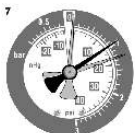
(7) READING: Reading slightly lower than normal including when throttle is suddenly opened then released. DIAGNOSIS: Worn piston rings. Carry out compression test.
