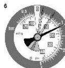
(6) READING: Regular fluctuation between normal and low. DIAGNOSIS: Blown head gasket between two adjacent cylinders. Carry out cylinder leakage test.
